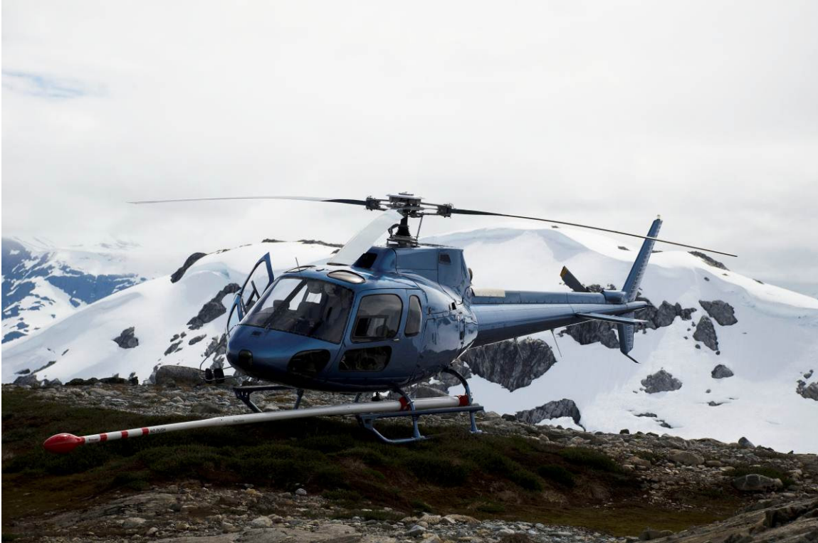
Figure 8: Eurocopter AS350 equipped with mag stinger for magnetic data acquisition, and internal spectrometer crystals for radiometric data acquisition.
