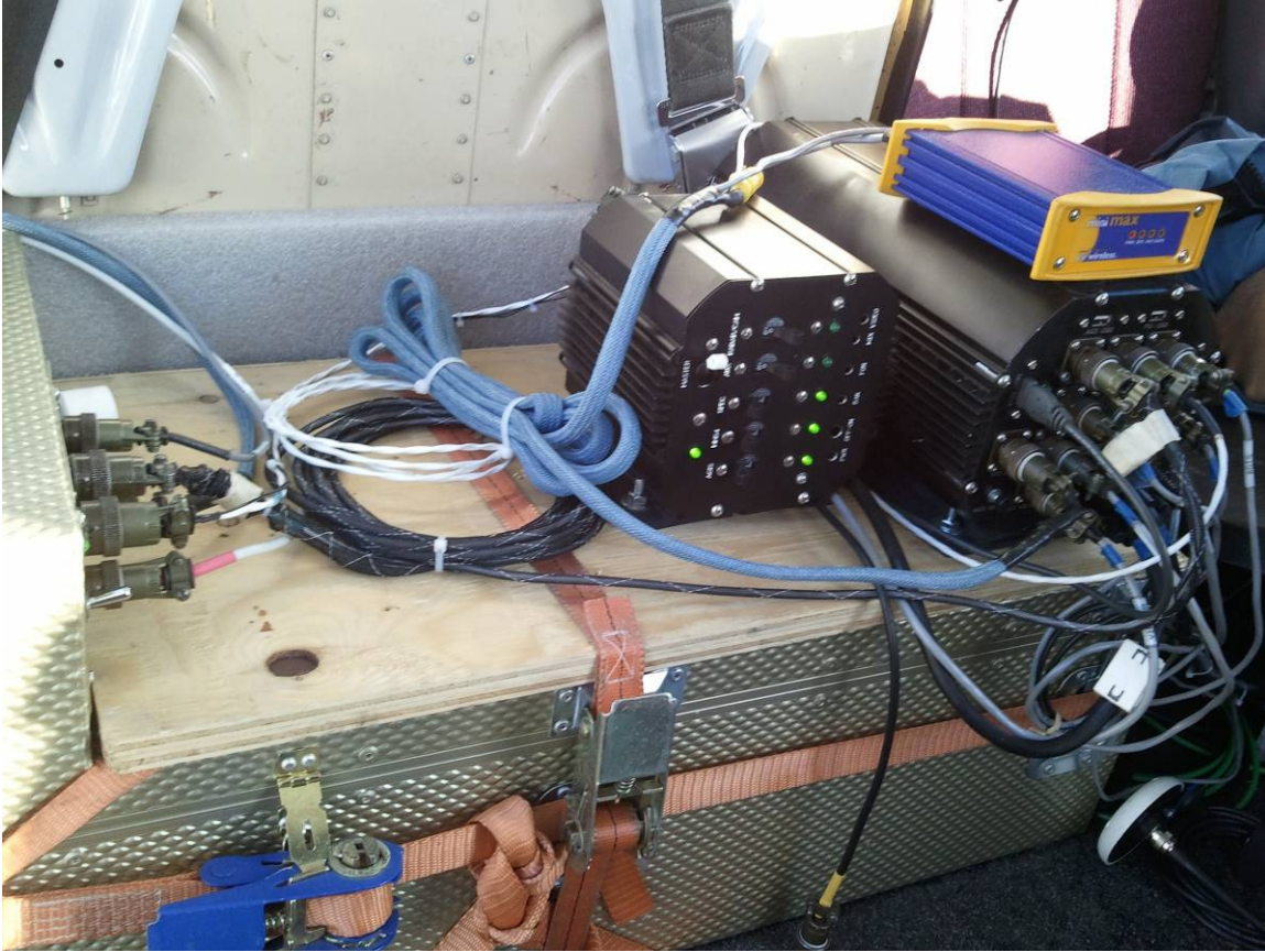
Figure 11: One of the IRIS strapped in the back seat of the Eurocopter AS350.
