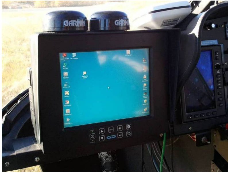
Figure 9: AGIS installed in the Eurocopter AS350.
